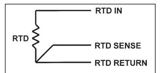
FIGURE 9-5. Three-Wire RTD Configuration.
